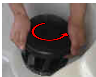
1. Swivel the protection grating anticlockwise.
