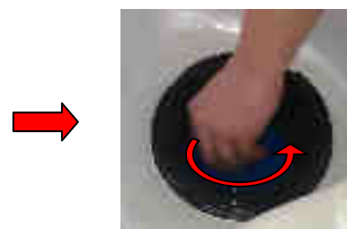
4. Swivel the paper filter anticlockwise.
